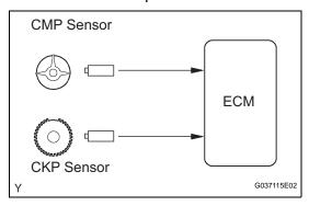
If the misfire exceeds the threshold levels, and could cause emission deterioration, the ECM illuminates the MIL and sets a DTC.
