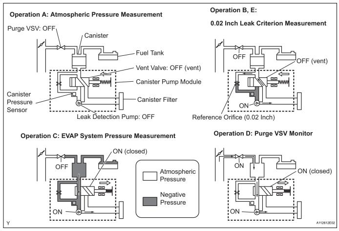
P0455: EVAP (Evaporative Emission) gross leak
