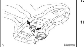
(diameter 3 to 4 mm (0.12 to 0.16 in.)) to the oil pan
