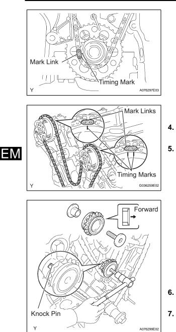
(b) Align the yellow mark link with the timing mark of the crankshaft timing link.
