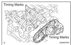
(b) Align the timing marks on the camshaft timing gears with the timing marks on the bearing caps, and install the camshaft timing gears with the chain onto the RH camshafts.
