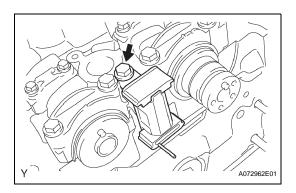
(b) Install the chain tensioner No. 2 with the bolt.
