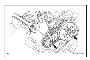
(d) Hold the hexagonal portion of the camshaft with a wrench, and tighten the 2 bolts.
