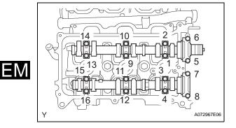
(f) Using several steps, uniformly install and tighten the 16 bearing cap bolts in the sequence shown in the illustration.
