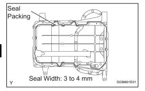
(c) Apply a continuous bead of seal packing (diameter 3 to 4 mm (0.12 to 0.16 in.)) to the oil pan as shown in the illustration.
