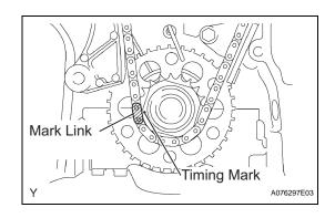
(b) Align the yellow mark link with the timing mark of the crankshaft timing link.
