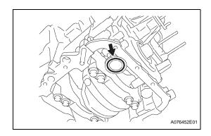
(b) Install a new O-ring onto the oil pump.
