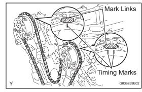
(c) Align the orange mark links with the timing marks of the camshaft timing gears, and install the chain.
