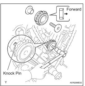
(b) Temporarily install the idle gear shaft No. 1 together with the idle gear shaft No. 2 while aligning the knock pin of the idle gear shaft No. 1 with the knock pin groove of the cylinder block.
