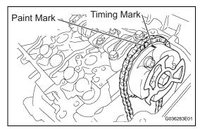
(k) Align the paint mark of the No. 1 chain with the timing mark of the camshaft timing gear.
