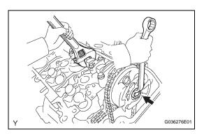
Hold the hexagonal portion of the No. 1 camshaft with a wrench, and tighten the camshaft timing gear set holt
