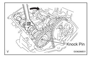
(f) Hold the hexagonal portion of the No. 2 camshaft with a wrench, and install the camshaft timing gear set bolt.
