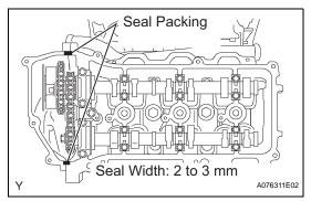
(b) Install the cylinder head cover within 3 minutes of applying seal packing. Tighten the cylinder head cover bolts and nuts within 15 minutes of installing the cylinder head cover. Otherwise, the seal packing mush be removed and reapplied.
