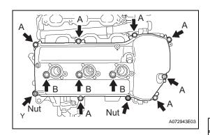
(d) Install the cylinder head cover with the 10 bolts and 2 nuts. Tighten the bolts and nuts uniformly in several steps.
