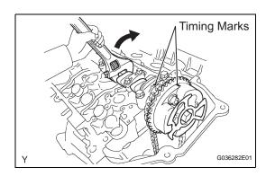
(j) Rotate the No. 1 camshaft clockwise using a wrench so that the timing mark of the camshaft timing gear is aligned with the timing mark of the camshaft bearing cap.
