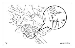
(f) Turn the crankshaft pulley 2 complete revolutions slowly until its groove and the timing mark "0" of the timing chain cover are aligned.
