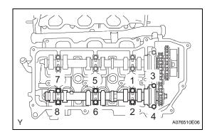
(d) Using several steps, uniformly install and tighten the 8 bearing cap bolts in the sequence shown in the illustration.
