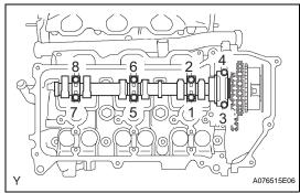
(i) Using several steps, uniformly install and tighten the 8 bearing cap bolts in the sequence shown in the illustration.
