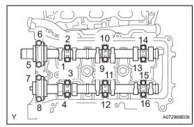
(f) Using several steps, uniformly install and tighten the 16 bearing cap bolts in the sequence as shown in the illustration.
