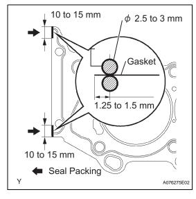
(c) Place the cylinder head gasket on the cylinder block surface with the Lot No. stamp upward.
