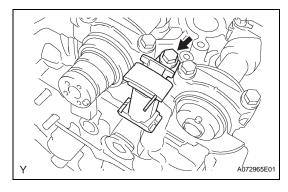
(b) Install the chain tensioner No. 2 with the bolt. Torque: 19 N\*m (194 kgf\*cm, 14 ft.\*lbf)
