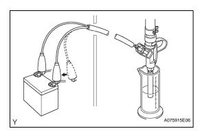
(16) Connect SST to the battery, then measure the injection volume for 15 seconds. Perform the inspection 2 or 3 times, then calculate the average.
