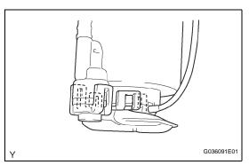
(b) Disengage the 5 claw fittings and separate the fuel pump from the fuel pump case.
