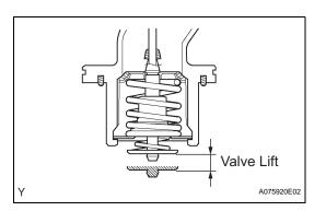
(c) Check the valve lift. Valve lift:
