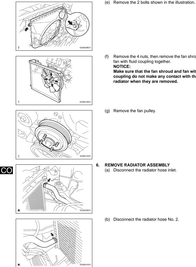
Remove the 4 nuts, then remove the fan shroud and fan with fluid coupling together. Make sure that the fan shroud and fan with fluid coupling do not make any contact with the radiator when they are removed.
