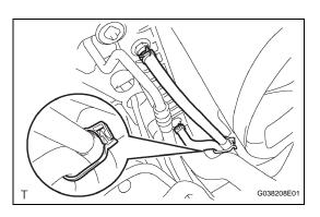
(d) Disconnect the oil cooler inlet and outlet hoses from the fan shroud. (for Automatic Transmission)
