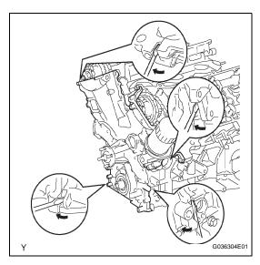
(b) Remove the timing chain cover by prying between the timing chain cover and cylinder head or cylinder block with a screwdriver.
