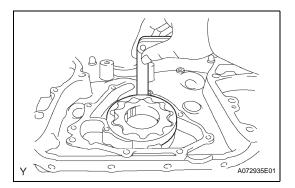
If the clearance is greater than the maximum, replace the drive and driven rotors. If necessary, replace the timing chain cover assembly.
