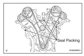
(d) Apply continuous beads of seal packing (diameter 3 to 4 mm (0.12 to 0.16 in.)) to the timing chain cover as shown in the illustration.
