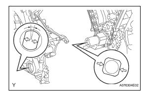
(e) Align the key way of the oil pump drive rotor with the rectangular portion of the crankshaft timing gear, and slide the timing chain cover into place.
