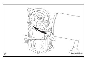
(b) Align the key of the starter yoke with the groove of the magnet starter switch.
