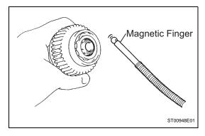
(c) Using a magnetic finger, remove the steel ball from the clutch shaft hole.
