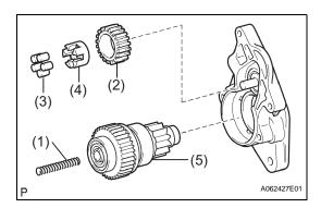
(b) Remove these parts from the starter drive housing.
