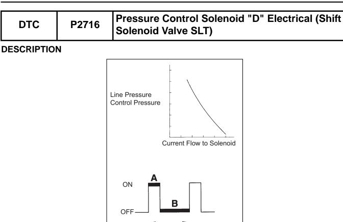
The linear solenoid valve (SLT) controls the transmission line pressure for smooth transmission operation based on signals from the throttle position sensor and the vehicle speed sensor. The ECM adjusts the duty cycle of the SLT solenoid valve to control the hydraulic line pressure coming from the primary regulator valve. Appropriate line pressure assures smooth shifting with varying engine outputs. Duty Ratio:
