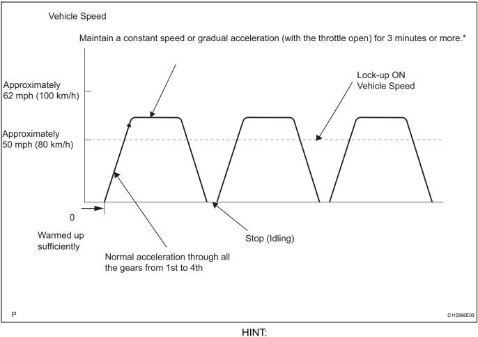
\*1: Drive at such a speed in the uppermost gear, so as to engage lock-up. The vehicle can be driven at a speed lower than that in the above diagram under the lock-up condition.
