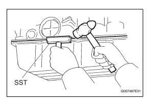
(b) Insert the blade of SST between the transmission case and oil pan, cut off applied sealer and remove the oil pan.
