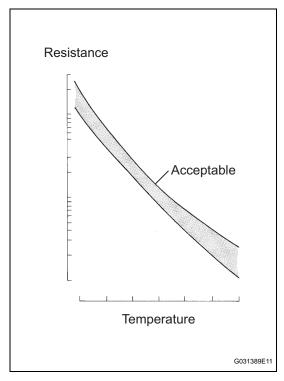
The ATF (Automatic Transmission Fluid) temperature sensor converts the fluid temperature into a resistance value which is input into the ECM.
