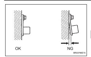
(a) Check the speed sensor (SP2) installation.
