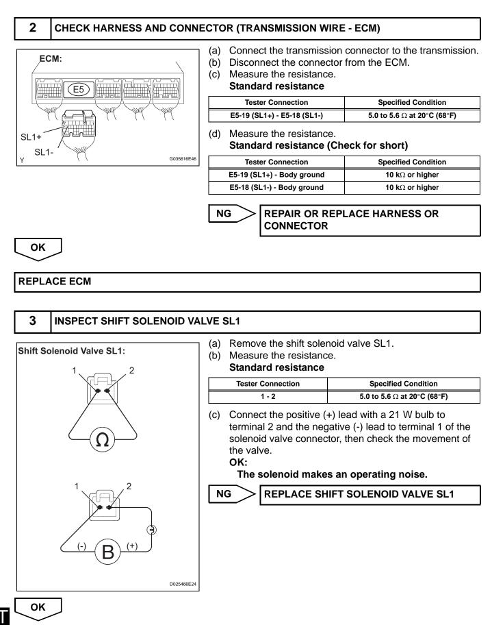
**REPAIR OR REPLACE TRANSMISSION WIRE**
