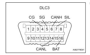
If the communication is normal when the tester is connected to another vehicle, inspect the DLC3 on the original vehicle.
