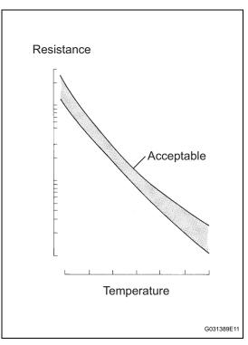
The ATF (Automatic Transmission Fluid) temperature sensor converts the fluid temperature into a resistance value which is input into the ECM.
