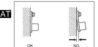
(a) Check the speed sensor (NT) installation.
