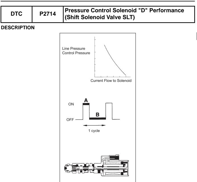
The linear solenoid valve (SLT) controls the transmission line pressure for smooth transmission operation based on signals from the throttle position sensor and the vehicle speed sensor. The ECM adjusts the duty ratio\* of the SLT solenoid valve output signal to control the hydraulic line pressure coming from the primary regulator valve. Appropriate line pressure assures smooth shifting with varying engine outputs. \*: The duty ratio is the ratio of the period of continuity in one cycle.
