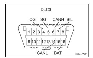
If the communication is normal when the tester is connected to another vehicle, inspect the DLC3 on the original vehicle.
