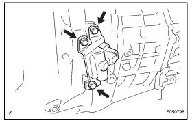
(b) Remove the 3 bolts and clutch accumulator.
