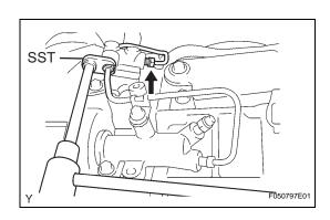
(c) Using SST, tighten the 2 flexible hose tubes.
