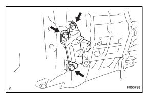
(b) Install the clutch accumulator with the 3 bolts. Torque: 12 N\*m (120 kgf\*cm, 8.7 ft.\*lbf)
