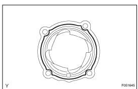
(c) Using a socket wrench (60 mm), provisionally tighten a new nut until there is no slack in the output shaft.
