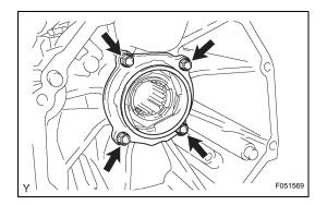
(b) Install the transmission case cover with the 4 bolts. Torque: 18 N\*m (184 kgf\*cm, 13 ft.\*lbf)
