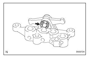
(b) Install a new E-ring onto the shift arm pivot.
