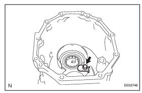
(b) Install the bearing lock plate with the bolt. Torque: 11 N\*m (115 kgf\*cm, 8.3 ft.\*lbf)
