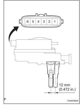
(a) Connect the wire harness side connector to the four wheel drive control ECU and inspect the wire harness side connector from the back side, as shown.
