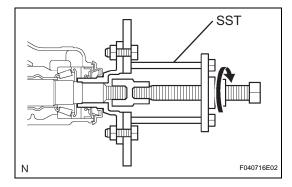
(c) Using SST to hold the companion flange, tighten the nut.
