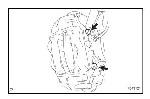
(c) Remove the 2 bolts and disc brake caliper.
