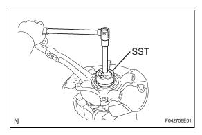
(b) Using SST, remove the front wheel adjusting nut. **SST 09318-12010**
