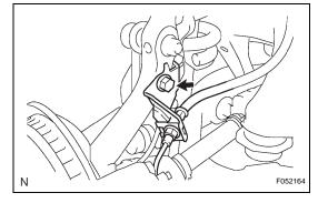
(b) Using SST, disconnect the brake tube from the disc brake cylinder.
