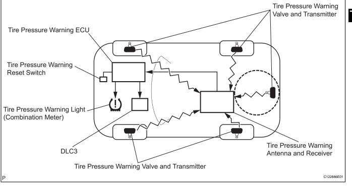
(b) After removing and installing the ECU or a tire pressure warning valve and transmitter, check that the normal code is output.
