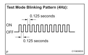
(e) Confirm that the tire pressure warning light in the combination meter blinks at 0.125 second intervals (4Hz).
