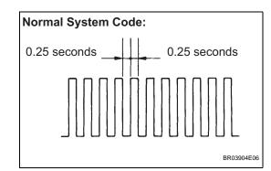
If 2 or more malfunctions are detected at the • same time, the lowest numbered DTC is displayed first.
