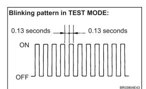
(g) Check that the ABS and VSC TRAC warning lights blink as shown in the illustration. HINT:
