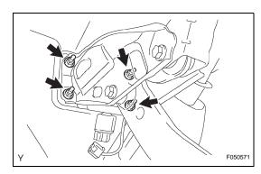
(b) Remove the 4 nuts, and pull out the brake booster.(c) Remove the gasket from the brake booster.
