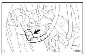
(b) Connect the oil pressure switch connector. **NOTICE:**
