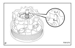
(c) Align the dent of the side plate with that of the vane pump housing front and install the side plate.
