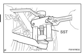
(b) Using SST, separate the tie rod end from the steering knuckle arm.
