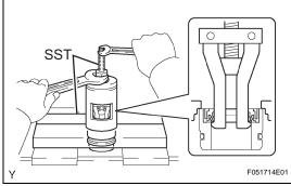
(c) Using SST, remove the rack bush oil seal. SST 09527-21011, 09612-24014 (09613-22011)
