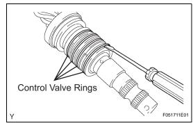
(g) Using a screwdriver, remove the 4 control valve rings.
