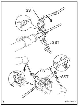
(b) Using 2 SSTs, remove the 2 steering rack ends and 2 claw washers.
