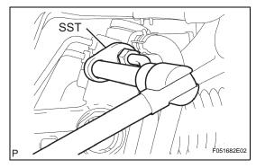
(c) Using SST, loosen the flare nut and separate the pressure feed tube.
