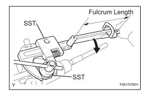
(c) Using SST, loosen the rack guide spring cap. **SST 09631-10021**
