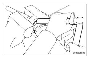
(I) Apply MP grease to the control valve as shown in the illustration.
