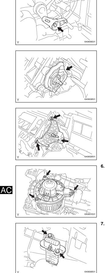
(g) Install the heater pivot with the bolt. Torque: 2.0 N\*m (20 kgf\*cm, 18 in.\*lbf)
