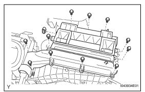
(b) Attach the evaporator top seal to the upper side and the evaporator bottom seal to the lower side of the evaporator.
