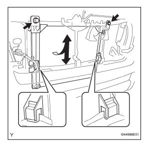
(e) Lift the condenser up from the rear side of the vehicle, and install the condenser lower brackets onto the upper part of the radiator lower supports with the 2 bolts.
