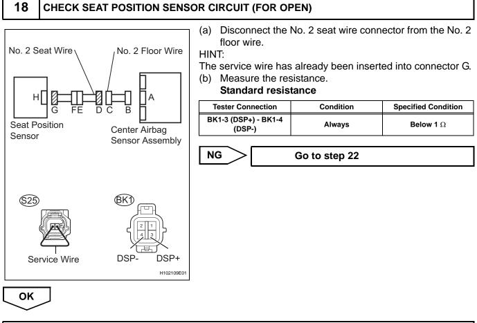
**REPAIR OR REPLACE NO. 2 FLOOR WIRE**
