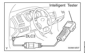
(4) Perform the zero point calibration by following the prompts on the tester screen.
