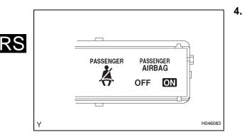
When the occupant classification system malfunctions, the SRS warning light comes on and the passenger airbag ON/OFF indicator indicates OFF. In this case, check the DTCs in the airbag system first.
