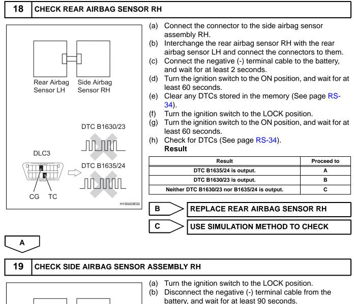
(c) Return the rear airbag sensor LH and RH to their original positions and connect the connectors to them.
