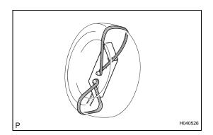
(3) Position the front seat side airbag assembly inside the tire with the airbag deployment side facing inside.
