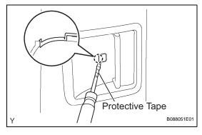
(b) Remove the screw, then remove the access panel inside handle bezel.
