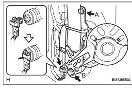
(e) Install the shoulder anchor with the nut.
