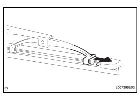
(b) Install the wiper rubber LH so that the head part (Larger side) of the wiper rubber faces the arm axle side.
