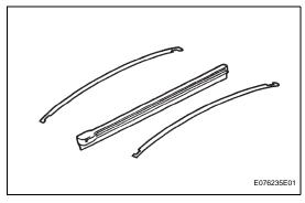
(b) Remove the 2 wiper rubber backing plates from the wiper rubber LH.
