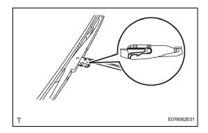
(b) Disengage the claw and remove the front wiper blade LH from the front wiper arm LH.
