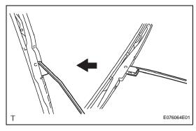
(b) Hold down the front wiper blade LH as shown in the illustration.
