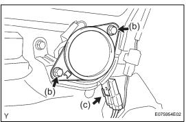
(b) Install the front No. 2 speaker assembly with the 2 bolts.
